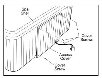
To replace the access panel, hold the access panel in place and secure it with the cover screws. **Be careful not to overtighten the screws.**
